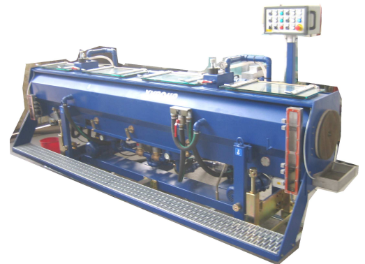
2 Chambers calibrating tank model BCV20-40 with closed circuit and plates heat exchanger For Pipes Ø max 200
