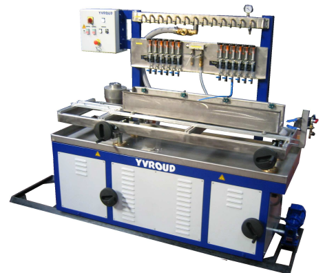
Profil calibration Table model BCP3000 Length 3 m – 3 pumps (1x vacuum + 2 x circulation)
