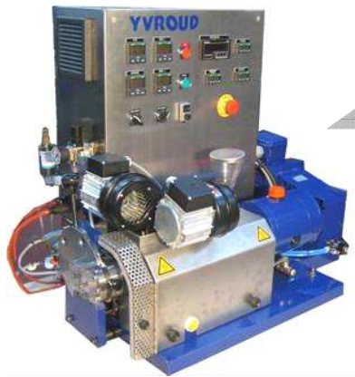
Laboratory extruder - diameters 16 to 30 mm
